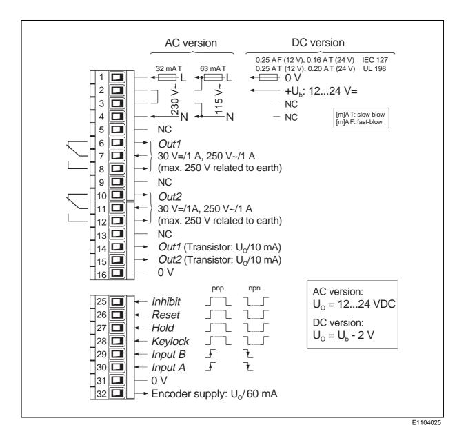
Note: The DC type has **no galvanic isolation** between the voltage supply and the electronic inputs and outputs!
